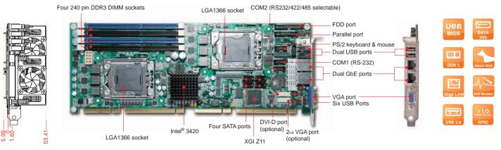
ROBO-8120VG2R is based on Intel® 3420 chipset and dual Xeon<sup>™</sup> processors. It's a server grade SHB built with high computing power and flexible PCI express expansion support, it's suitable for military, industrial automation, and digital signage applications.
